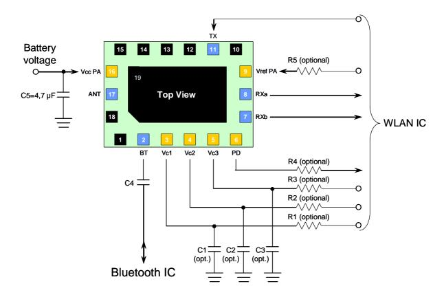
All RF ports are 50 Ohm matched. WLAN RX ports are matched to 100 Ohm differential impedance.
