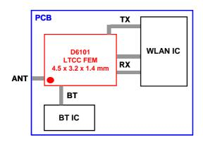
The D6101 front-end module is intended for mobile phone applications, where size is a critical parameter.
